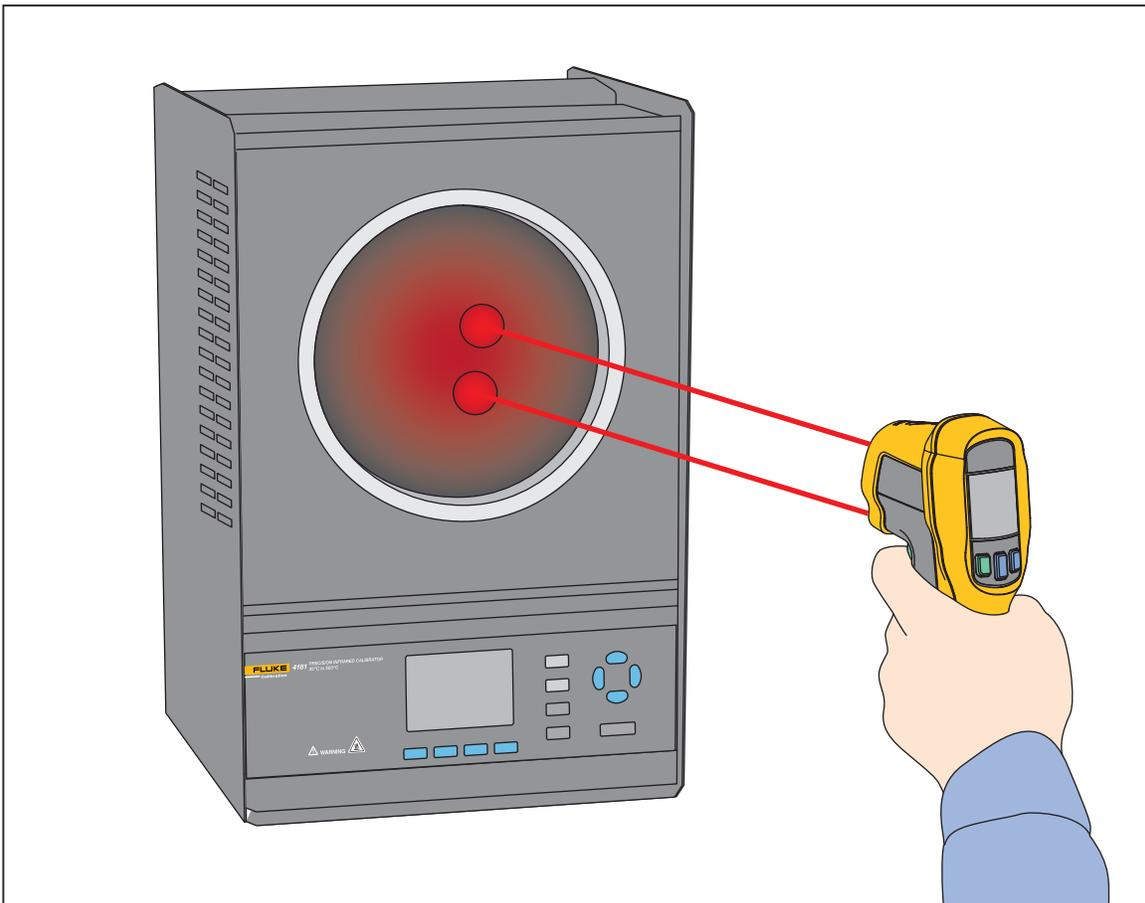
**Figure 3. Aim the 62 Max + for Verification**
